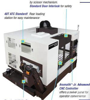
Standard Lift Up Conveyor can be positioned on either left or right-hand side of the machine
