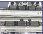
**3-Block, Double Roller LM Guide System**Ultra-super-high rigidity.
