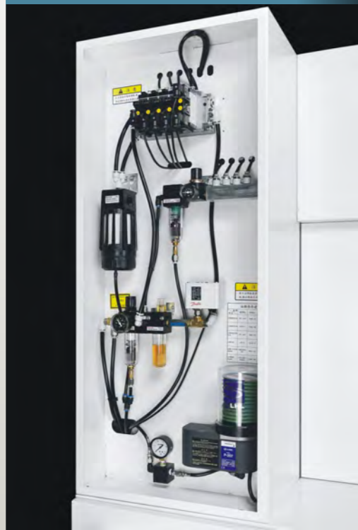
Pneumatic and Lubricant system
