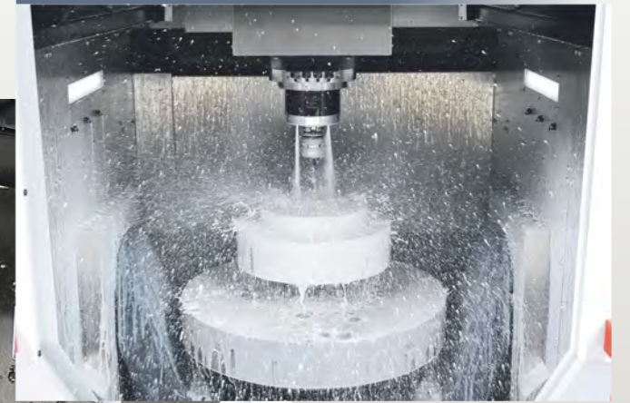
Circular water Flushing System
